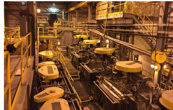
Existing Flotation Circuit
