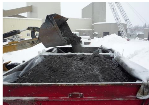
Concentrate being loaded for shipment to Sudbury
